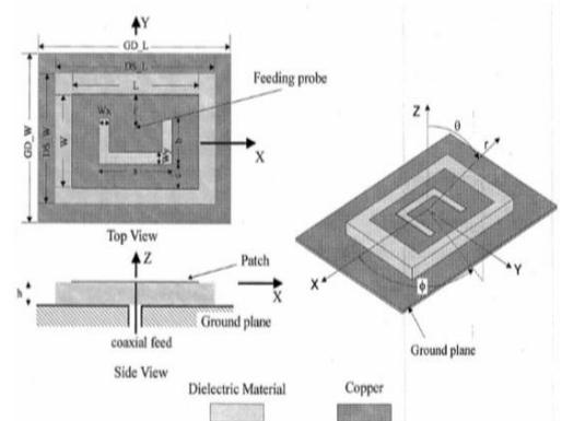
Fig 5. Geometry of a U-slot rectangular patch antenna printed on a microwave substrate.
