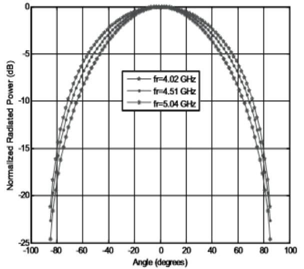
Fig 11. Variation of radiation pattern different frequencies
