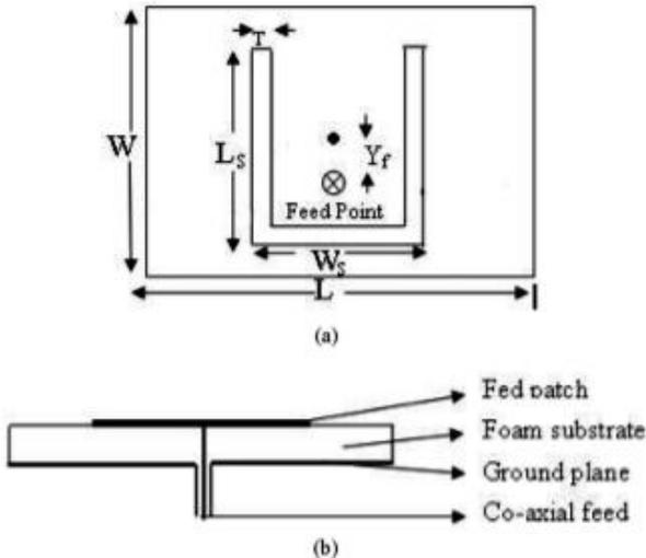
Fig 10 (a) Top view of the proposed antenna, (b) Slide view of the proposed antenna
