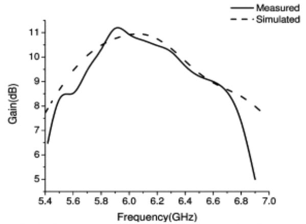
Fig.3. The simulated and measured gain of  $2 \times 2$  array.
